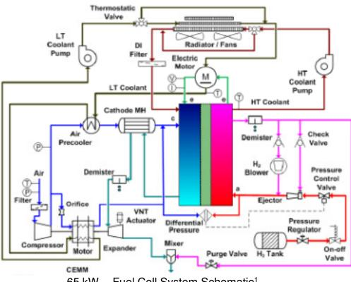
65 kW<sub>net</sub> Fuel Cell System Schematic<sup>1</sup>
