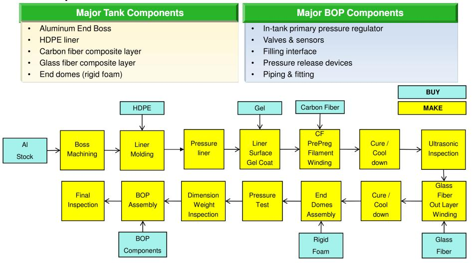
PEMFC Plug Hybrid Vehicle On-board Compressed H2 Storage System *Preliminary Cost Results* In the 5,000 PSI baseline system, the carbon fiber composite layer was the dominant cost driver.
